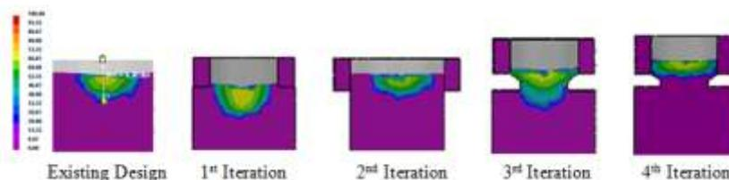
**Shrinkage porosity in feeder zone of existing design and new designs**
